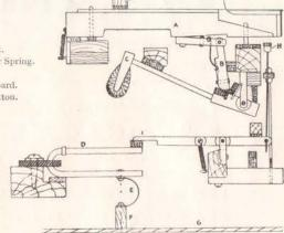
On depressing the key (A) the jack (B) causes the hammer (C) to strike the tuning fork (D) and produce the sound, which is reinforced by passing through the semi-circular spring (E) to the bridge (F) and thence to the sounding board (G). At the same time the front of the key depresses the damper button (H) causing the damper (I) to lift clear of the tuning fork, which is then free to vibrate.
